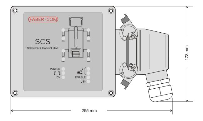
The SCS device is a stabilizers control unit integrated with some auxiliary functions useful for the control of cranes installed on trucks. The core of the unit is a microprocessor based electronic card for the advanced control of the machine, which makes available in one device the following features:
