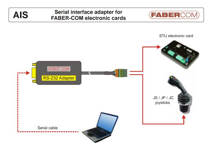
The AIS Serial Interface Adapter is the only medium to connect FABER-COM electronic devices (STU electronic card and JS/JP/JC joysticks) to a PC for programming, calibration, firmware updating and working parameters monitoring.
