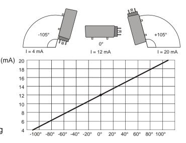
Attention: the input resistance of the used instrument (for the measurement) must have a value that allows to the sensor to supply the maximum current.
